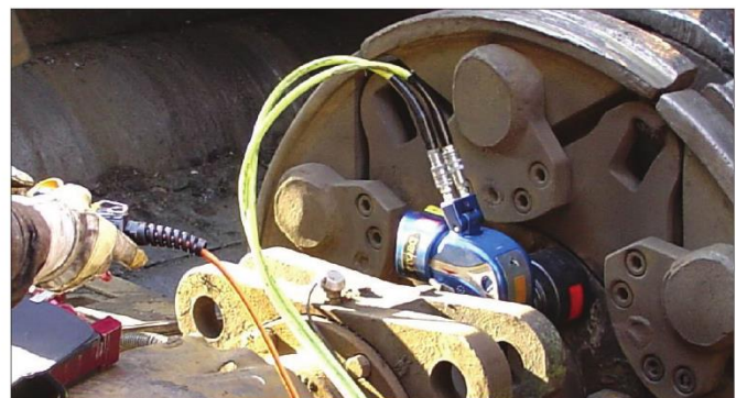
MXT-10 being used on a scrap press
